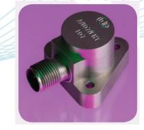
Industrial grade vibration transducers high temperature 10pC/g version is rated to 400°C. Signal output is floating, via 2 pole hermetic connector, thus minimizing common mode interference. Ingress of contaminants into the transducer and/or connector will degrade data. Transducers and cables can be supplied proof pressure tested to 80bar, individually and as assemblies.
